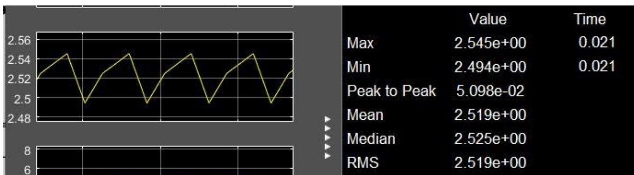
Figure 34: SEPIC converter inductor ( L_2 ) ripple current graph
